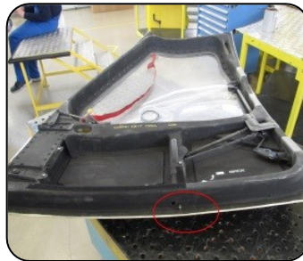
Loose sleeve left by manufacturer in helicopter door
